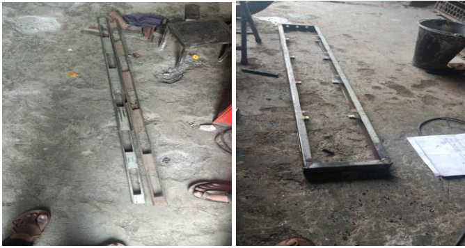
Fig-17: Fabrication of truck chassis
